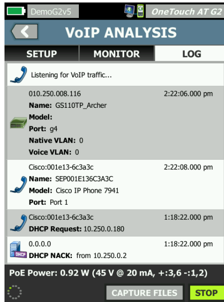
Figure 28: VoIP Analysis shows the entire call setup process as well as quality of the VoIP call in each direction.
