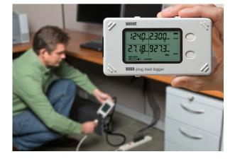
**Supported Measurements:** RMS voltage, RMS current, active power, active energy, apparent power, and power factor
