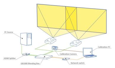
B. Please follow Smart Planner drawing guidance for projector and camera installation. Adjust projection position adjustment, zoom & focus as required. The real projection area MUST be larger than desired display dimension.
