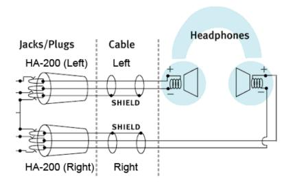
In the 'Balanced Headphone Mode', simply use the XLR input (one on each HA-200) and output.
