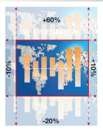
MOTORIZED LENS SHIFT Horizontal: ±10% Vertical: -20% +60%
