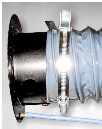
Figure 5. Connecting Pressure Tubing to Tap on Primary Duct Adapter. Bung not shown.
