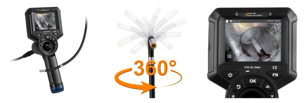
4-way industrial borescope with photo and video recording / 1280 x 720 pixels / 360° swivel / 6 mm (0.23") diameter / 1 meter (3 ft 2") cable length / LED lighting / Micro-SD card memory / Transport case / Battery life >3 hours / IP 67
