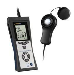
used for outdoor measurements in sunlight and testing at workplaces with high light requirements. The spectral sensitivity of the light meter is adapted to the brightness sensitivity of the human eye in daylight.
