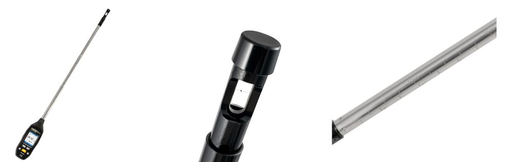
Environmental meter with data memory / Measuring range 0 ... 30 m/s (98 ft/s) / Micro-USB interface / 3/8" tripod mount / CSV file format / Rechargeable battery / Optional with calibration / Telescopic probe extendable up to 426 mm (16.7")
