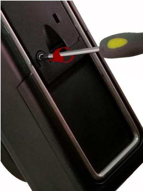
Step 1 - Remove security screw with Phillips screwdriver
