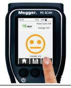
The current measurement screen is saved as a **screenshot.** A keypad for entering the file name appears. Pressing the button saves the screenshot in the data folder for the current measurement. The software then immediately returns to the measurement screen.
