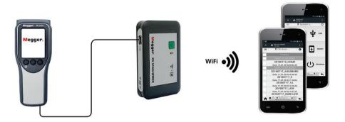
When a PD scan is connected to the WMDS, all new measurement data sets are automatically downloaded to the internal memory of the WMSD. This function means that the mass storage device can also be used to collect the measurement data from multiple measuring devices that are in use without having to bring them to the office.
