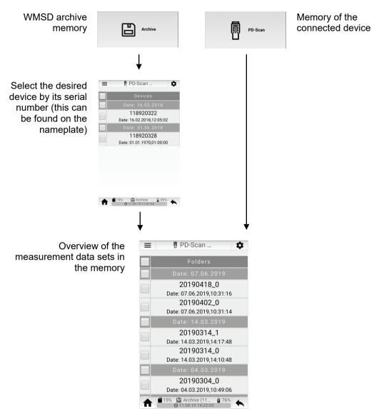
All measurement data stored in the memory of the connected PD Scan should also be stored in the archive database once the automatic data transfer is complete. However, the measurement data on the connected device can usually be located more quickly in the device's memory as it normally contains fewer data sets and the device does not need to be selected as described above.
