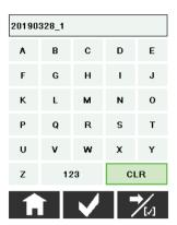
Briefly pressing the button allows the user to scroll through the list of fields on the touch screen. Pressing the button deletes the last character that was entered. Pressing and holding the button deletes all characters. You can switch to the numeric keypad by pressing 123. In addition to number keys, the keypad also has six freely assignable keys for frequently used text modules.
