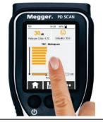
The measurement is paused and the current measurement results are frozen. If headphones are connected to the device, then the acoustic, audible signal is also muted. Instead of the button, the button used to continue the measurement now appears at the bottom edge of the screen. Briefly tapping the display again also allows the measurement to be continued.
