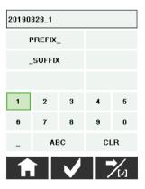
Briefly pressing a text module adds it to the end of the current character string. Pressing and holding the text module opens it for editing.
