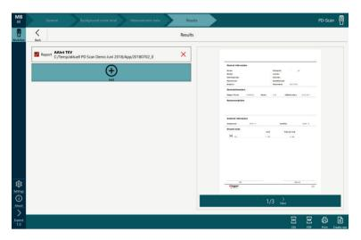
Should there be any other measured data folders for the same measurement object, which are relevant for the report, then they can be added to the report using the  $\bigoplus$  button. If there are several measured data folders, then the order in which they appear in the report can be changed using drag-and-drop.
