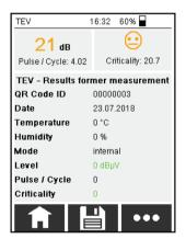
This screen allows you to quickly and reliably identify whether the measured values have, for example, worsened in comparison to a measurement performed 6 months ago.
