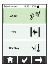
Pressing the required field on the touch display, or navigating to the required field using , followed by , allows the required operating mode to be started.
