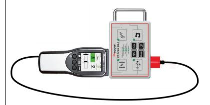
Since a bar deflection only takes place above 10 dB, the setting **High** must be selected using the **Lev** button in this operating mode!
