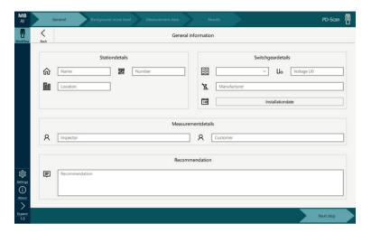
This menu allows general information about the station, the measurement itself and recommended action based on the measurement results to be entered.
