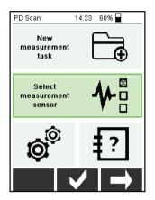
Pressing the **Select measurement sensor** field on the touch display or pressing vopens the menu for selection of the operating mode.
