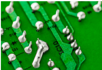
PCB and solder joint inspection
