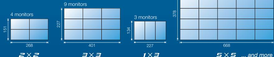
Almost any number of PN-V600A/PN-V601A monitors may be joined together to create high impact multi-screen video walls. These configurations may be controlled through RS-232C or over a network.\* Their ease of control and ease of integration help simplify the design and installation of sophisticated video wall displays of most any size and shape.
