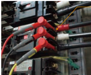
Magnetic design (diameter: 11 mm)
