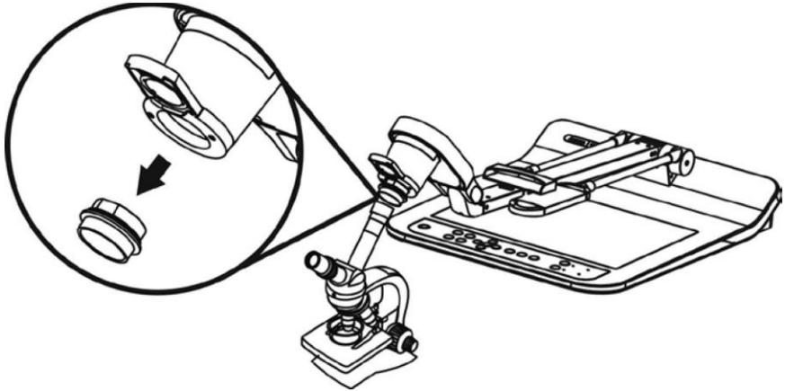
For eyepieces of  $\text{Ø}28$  mm or  $\text{Ø}31$  mm, fit one microscope adapter with the greatest diameter along with another appropriate one.
