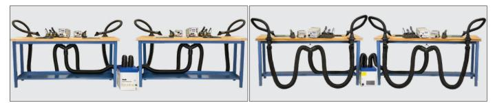
Arm-Evac 200 or 250 (Arm-Evac 250 shown. See pages 4-5 for specifications.) Four 50mm (2") diameter, 36" long, ESD Flex Arms: P/N 8882-0435-P1 Two 50mm (2") Bench Mounting Kits: P/N 8886-0553-P1 Two Bench Mounting Brackets: P/N 8886-0552-P1
