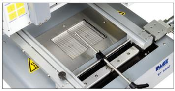
To prevent sagging/warping during reflow, an integrated Board Support Wand is used on the TF1800 (shown above), while the TF2800 includes an innovative Board Support Beam.
