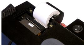
Feed the paper through the the paper slot in the cover (using the paper feed button on the hand-held unit).
