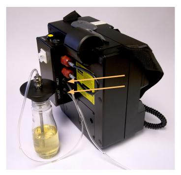
To fit a hose or plug, push into the fitting until the seal resistance is overcome.
