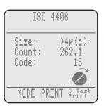
NOTE: The minimum and maximum ISO codes that can be measured are 7 and 22 respectively. If the result is below 7 then '0' is displayed; if the result is above 22 then '99' is displayed.
