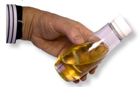
**DO NOT SHAKE the fluid sample** at this stage as this will introduce air in the fluid and lead to poor results. A gentle tumbling action is required.
