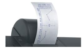
16-column printer for hard copy data. A feature of the icountLCM is the on-board printout data graphing option developed to support predictive maintenance procedures.
