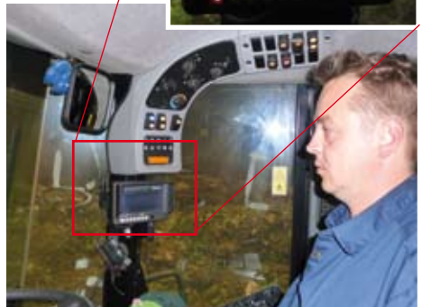
The thermal images of the FLIR Systems PathFindIR are displayed on the same LCD as the images of the reversing camera. Note the hot spot in the thermal image which clearly shows a part of the waste pile that was turned.
