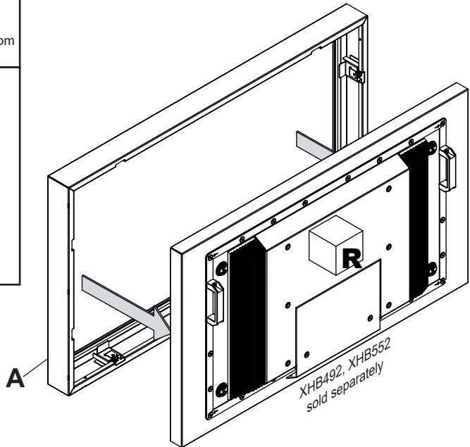
[ENG] Drainage holes indicate bottom of overlay.
