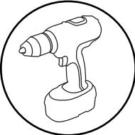
⚠ To properly tighten screws: Tighten until screw head makes contact, then tighten another 1/2 turn. Do not overtighten screws.
