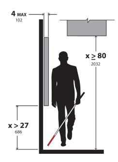
4 inches from the wall and a minimum height of 27 inches with a maximum height of 80 inches.
