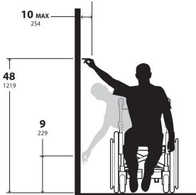
It is also important to remember the ADA requirement for the blind and partially sighted, which is concerned with the kiosk being easily detectable by a cane. If a kiosk is mounted on the wall, it is required to have a maximum depth of
