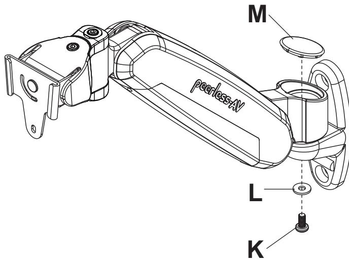
5 Hook adapter plate onto arm assembly (B).
