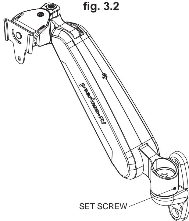
4 Secure arm assembly (B) to wall plate (A) with one M6 x 12mm phillips screw (K), one M6 plastic washer (L), and cover (M).
