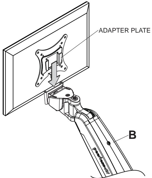
7 Cables may be routed using cavity in arm assembly (B). Remove the cable cover on arm assembly (B) by pressing firmly in the middle of the cable cover and then pulling the flanges of the cable cover. Route the cables in arm assembly (B) and then reinstall the cable cover.
