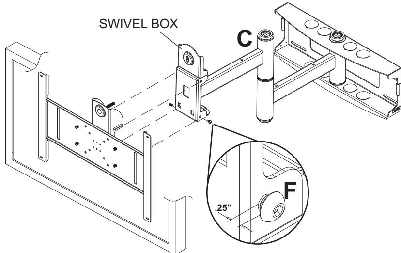
6-1 Hook tilt-roll assembly (B) onto M10 screws (F). Insert carriage bolt (I) into slot of swivel box as shown in figure 6.1. Install nylon washer (G) and tilt adjustment knob (H).
