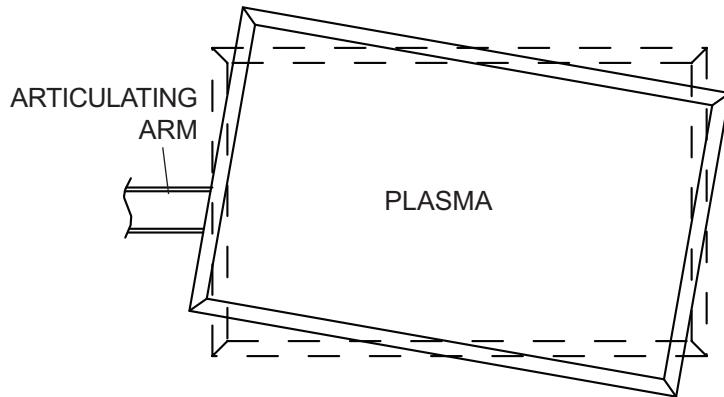
**7-1** If it is too difficult to adjust roll of plasma, loosen screws shown in figure 7.1 using a phillips screwdriver.
