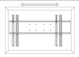
Secure displays by tightening adapter bracket screw.
