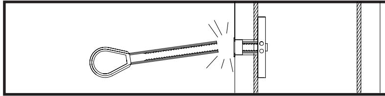
**4** Attach wall plate (A) with 1/4-20 x 2.5" phillips screws (C), and washers (E).
