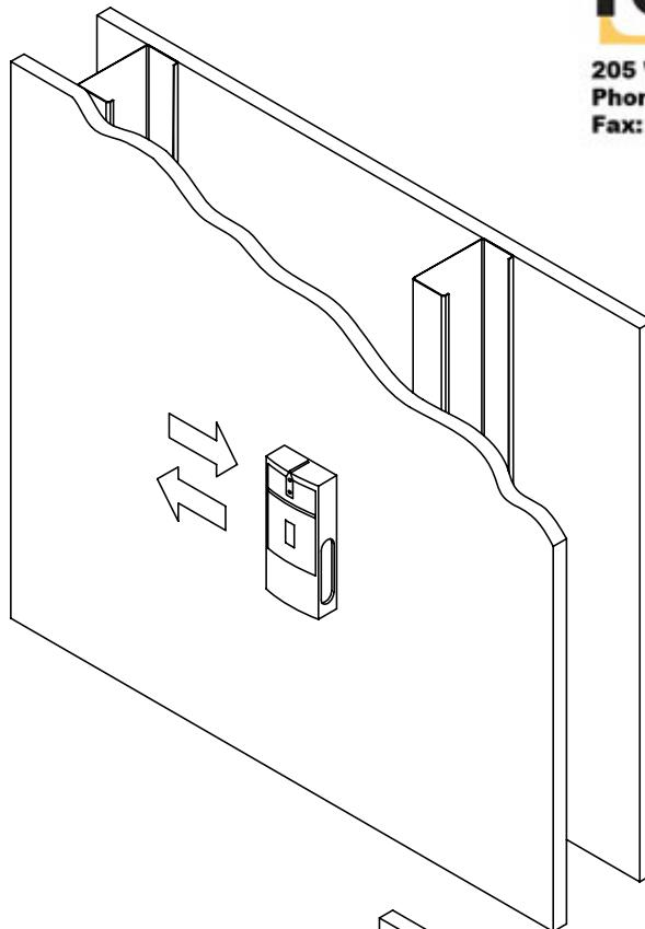
2 Use wall plate (A) as a template to mark slot centers on stud centers.
