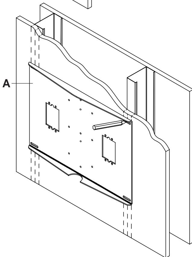
**3 FOR METAL STUD WALLS ONLY:** Drill four 1/2" (13 mm) dia. holes through drywall and studs. Insert togglers (D) as shown below...
