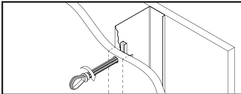
**3-4** Slide plastic cap forward while pulling back firmly on ring.
