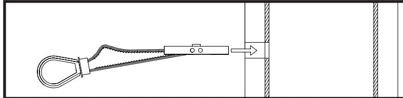
**3-3** Rotate toggler clockwise to wedge it against inside walls of metal stud.
