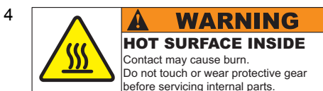
This label warns users that they risk being injured if their hands come into contact with a hot surface: wear protective gloves before any intervention.
