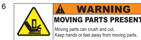
This label warns users about the risk of crushing or cutting due to moving parts: keep a safe distance and/or keep your hands away from the moving parts.
