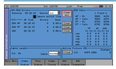
The Video Status menu display the status of the selected video input and displays any errors that have been found in the data stream.
