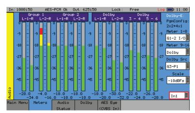
If the Dolby metadata analysis option is installed then the audio levels defined in the metadata can be displayed on the meters.
