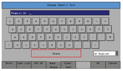
When editing text, the keyboard above is displayed to allow easy editing. Move the cursor to select the key to 'press' and then press 'Ok' to 'press' it. The Shift menu key causes the next keyboard to change to shift mode for the next key press.
