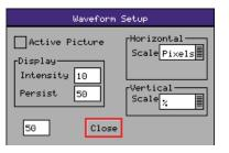
The Waveform Setup menu allows the vertical and horizontal scale of the waveform display to be setup as well as controlling the intensity and persistence of the display.
