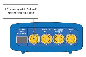
In this example, the SDI signal contains embedded audio with Dolby-E present on one or more audio pairs. The Sx instrument needs to lock its internal audio clock to the SDI signal (Generator – Genlock – Source = Input 1) and the Dolby Timing source should be set to SDI.
