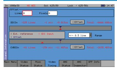
The Video Timing menu displays the relationship between the SDI and composite video inputs with respect to the locking reference input.
