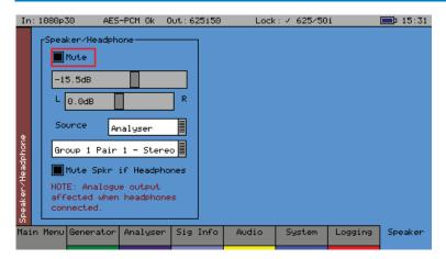
The Speaker menu controls which audio pair that can be heard on the loud speakers and headphone output of the unit. Menu Reference
