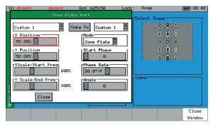
The Programmable zone plate option (PHSXOZ) adds a range of pre-programmed zone plate patterns along with user defined controls over several parameters which can be saved to custom buffers.
