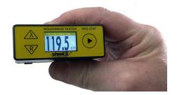
The SRG-2200 determines surface roughness parameters Ra, Rz, Rq and Rt within a wide measuring range. The piezo-electric pick-up stylus with diamond tip assures a very reliable measurement within tolerances that conform to ISO class 3. Roughness parameter Ra is computed to conform to ISO and Rz is computed to conform to DIN.
