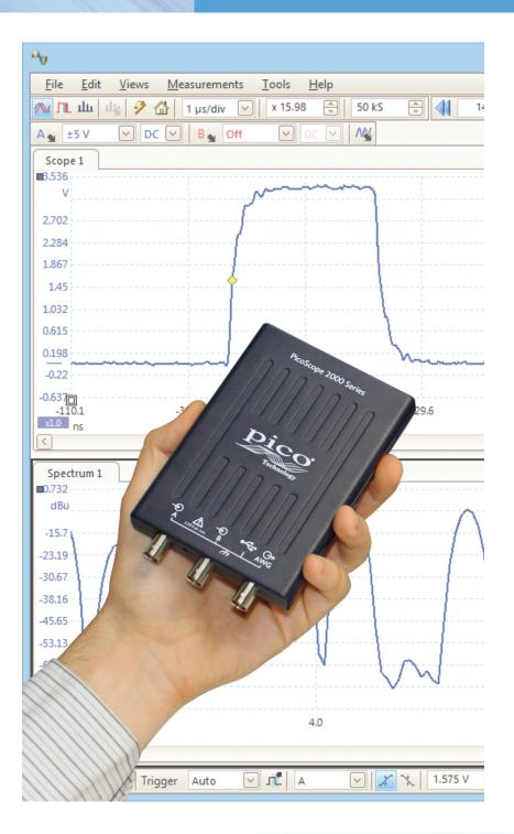
2 channels Low cost 200 MHz bandwidth Up to 1 GS/s sampling rate Arbitrary waveform generator Advanced digital triggers Persistence display modes USB connected and powered Mask limit testing Serial bus decoding
