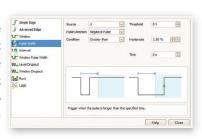
All triggering is digital, resulting in high threshold resolution with programmable hysteresis and optimal waveform stability.
