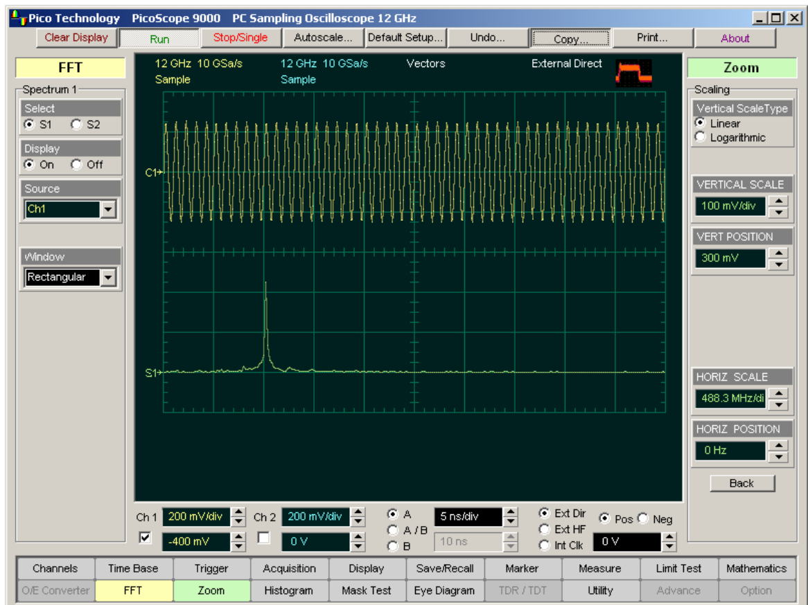
The 1-GHz sine-wave signal shown in both the Time Domain and the Frequency Domain
