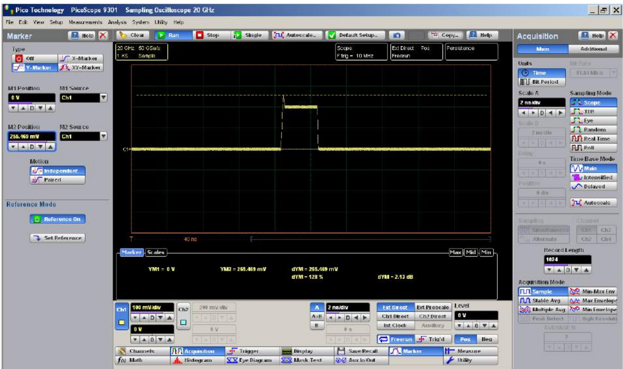
Ratiometric measurement of Overshoot with Y Markers
