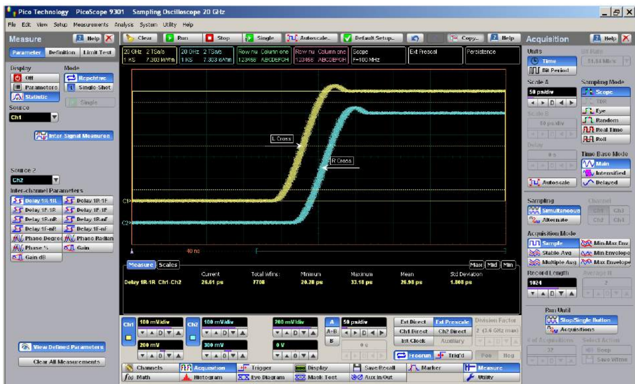
Two waveforms with entered deskew of 27 ps
