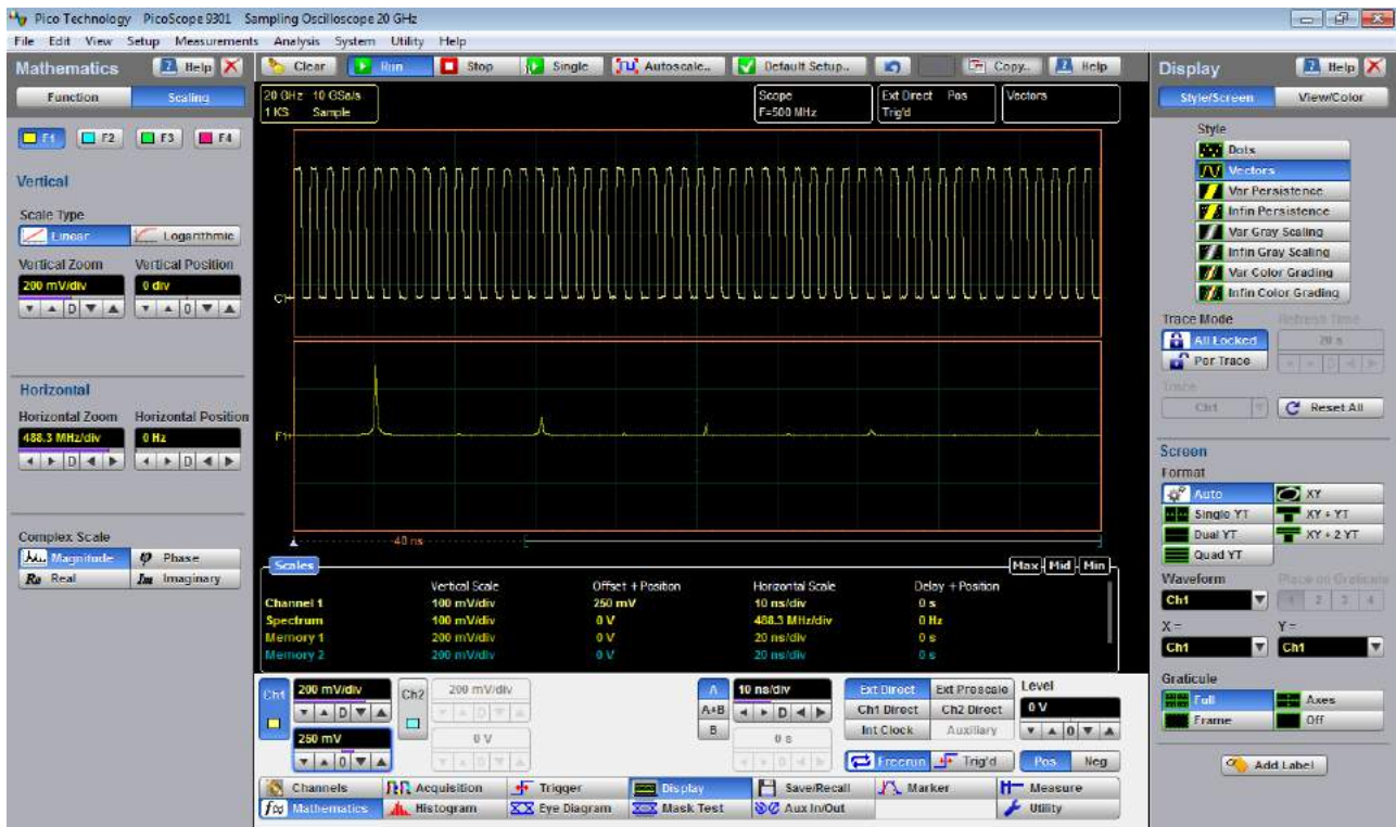
Spectrum Magnitude of 500 MHz pulse waveform
