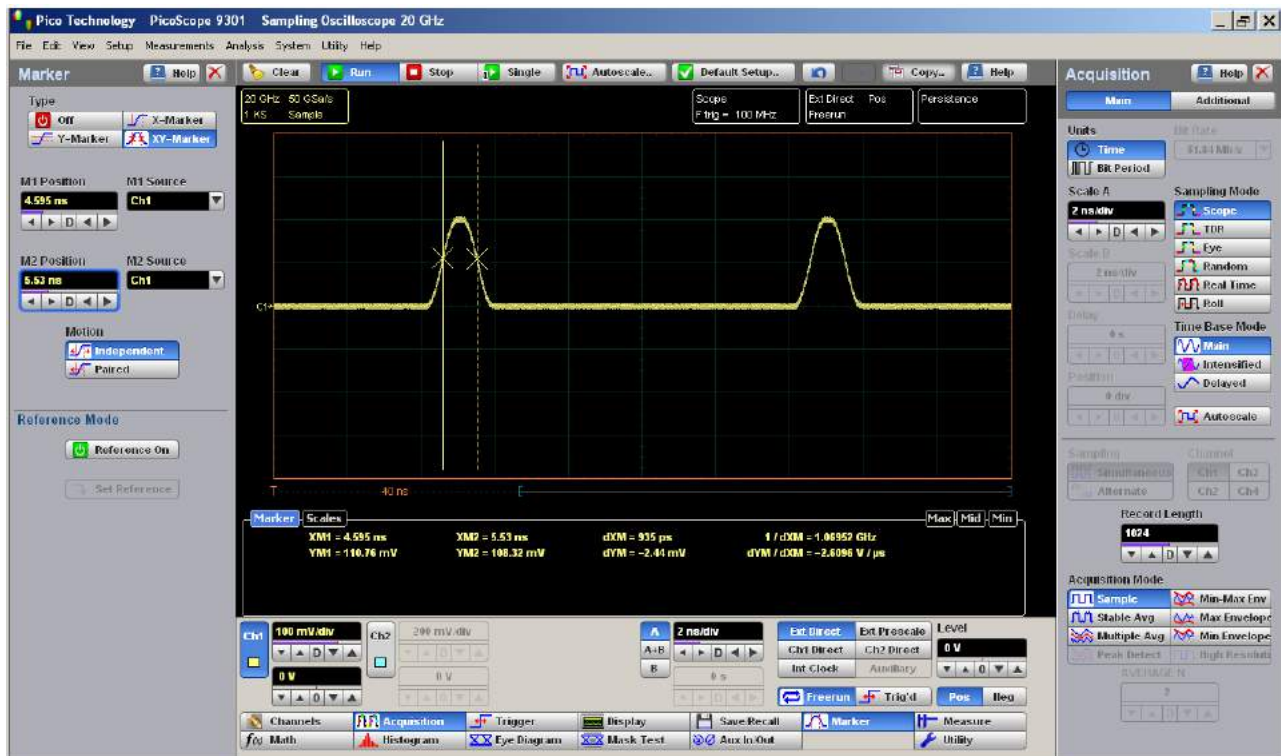
Customized measurement with the XY Markers
