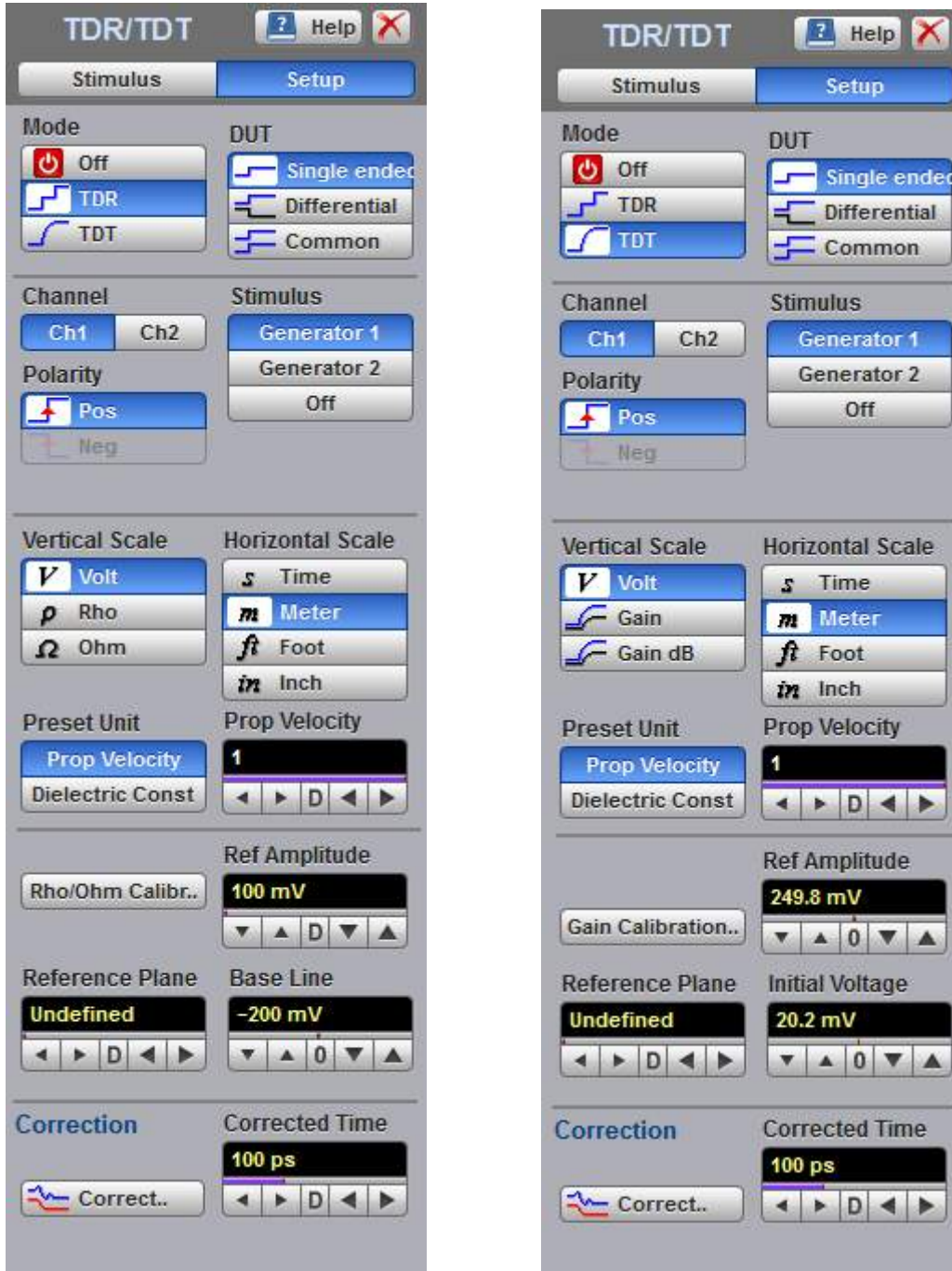
TDR/TDT Setup menu for PicoScope 9311/9312 oscilloscopes in TDR mode (left) and TDT mode (right)
