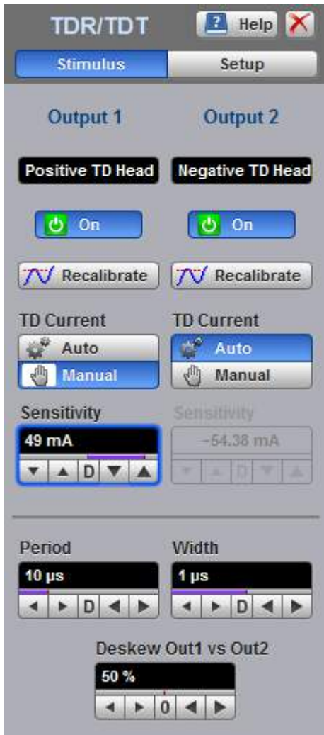
TDR/TDT Stimulus menu for PicoScope 9312 oscilloscope
