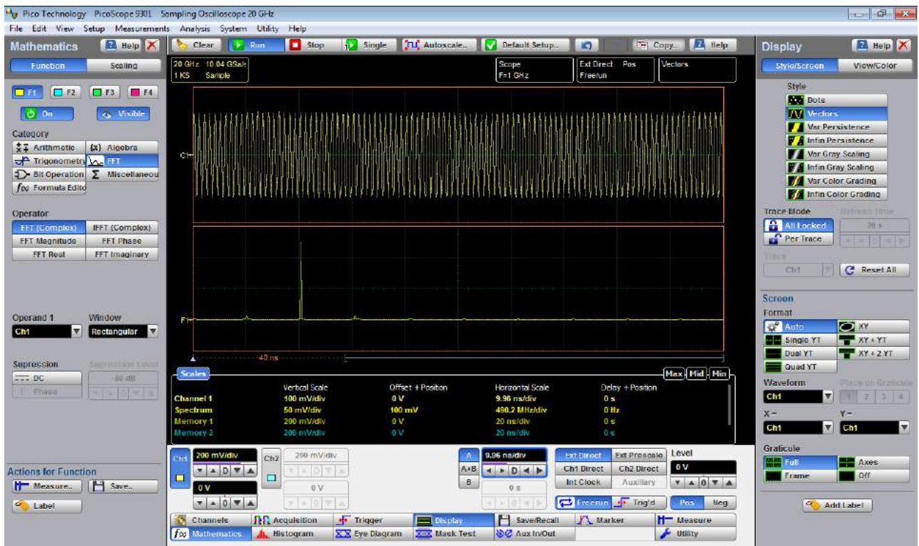
FFT having small amount of leakage
