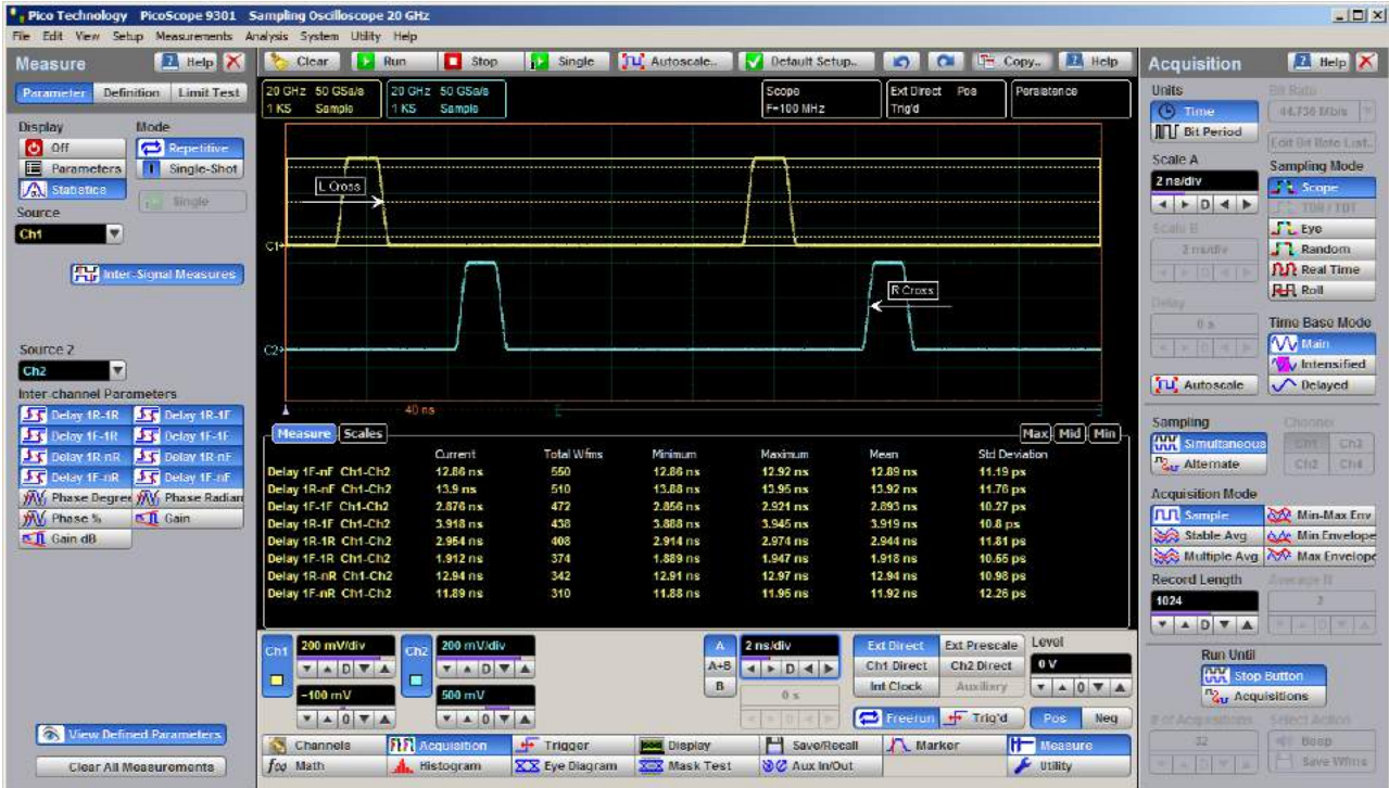
Example of Delay measurement between two waveforms
