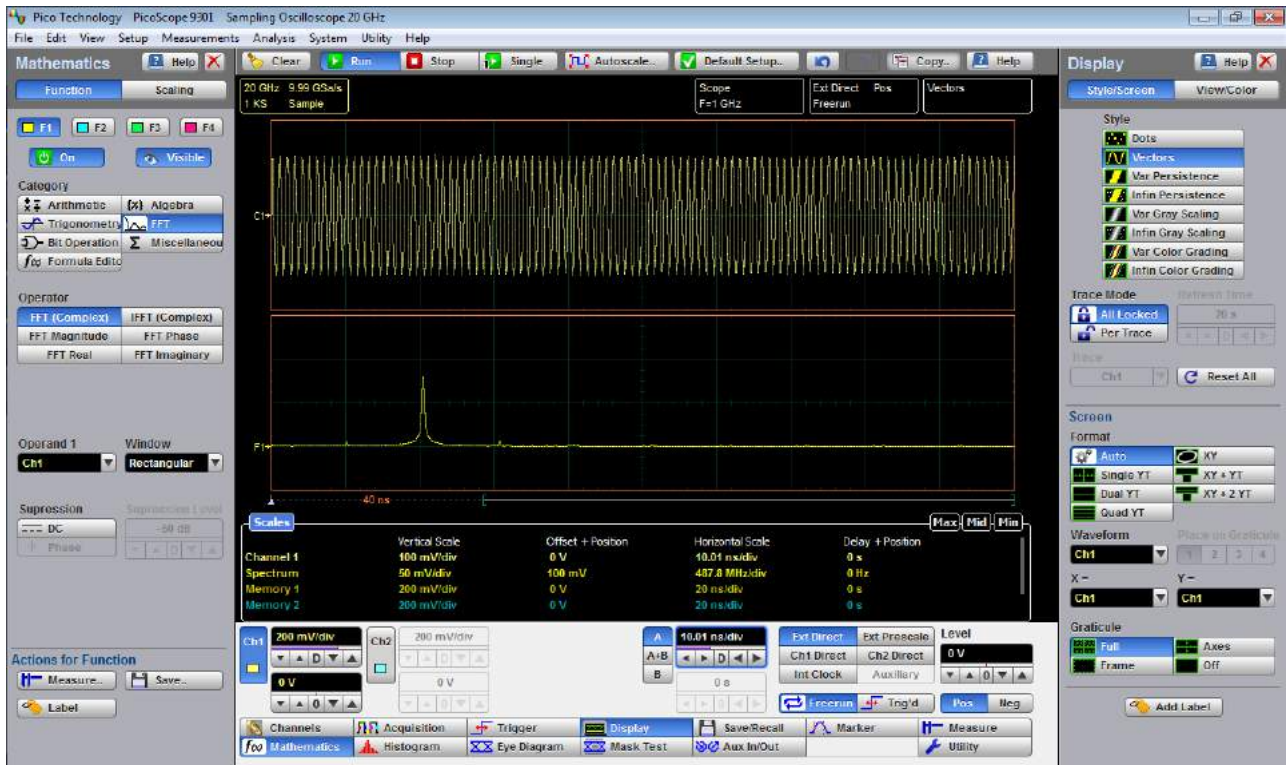
FFT with leakage
