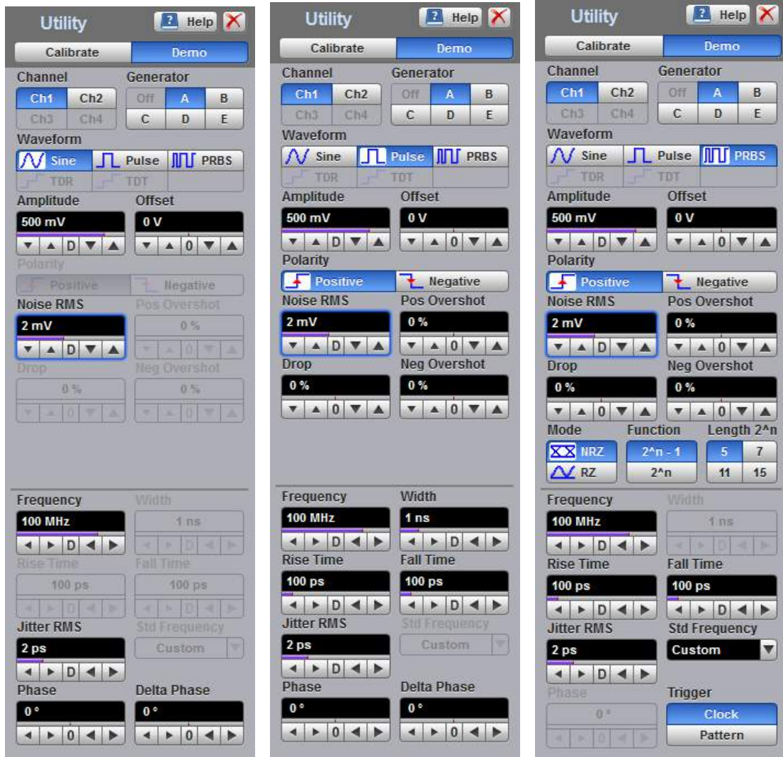
Utility menu with Sine, Pulse, and PRBS waveform options selected
