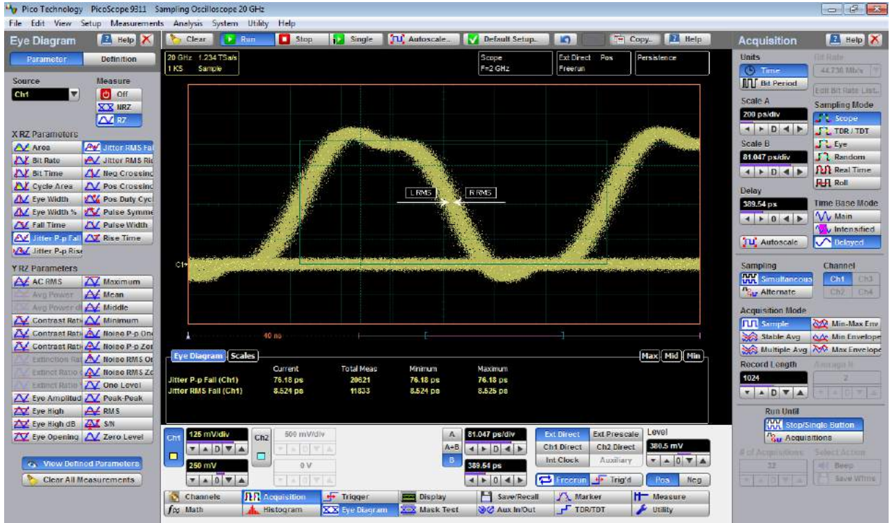
RZ Jitter P-p, Fall and RZ Jitter RMS, Fall definition
