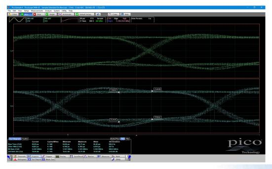
Eye diagram analysis can display data including: bit rate, period, crossing time, frequency, eye width, eye amplitude, mean, area and jitter RMS. Also shown on the graph are left and right RMS jitter markers. These measurements are selectable from within the Eye Diagram side menu and are listed on screen below the graph.
