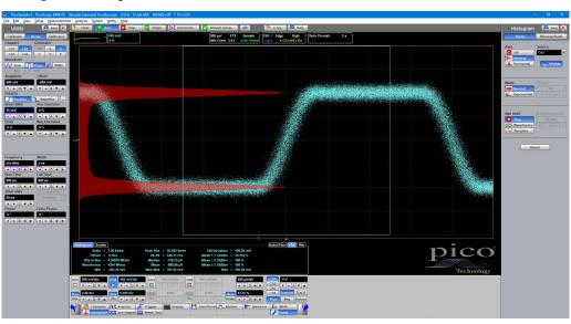
Behind the powerful measurement and display capabilities of the 9400 Series lies a fast, efficient data histogram capability. A powerful visualization and analysis tool in its own right, the histogram is a probability graph that shows the distribution of acquired data from a source within a user-definable window.
