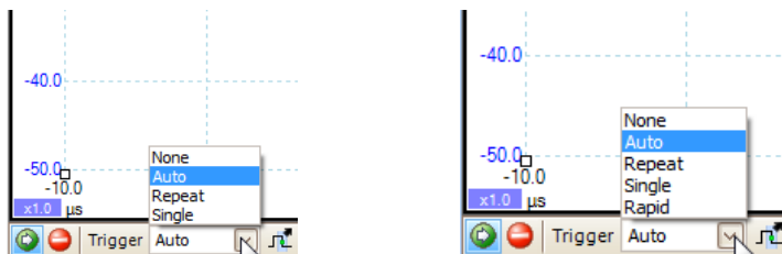
The Triggering toolbar before and after enabling Spectrum and Persistence modes
