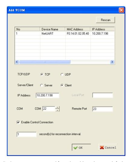
Select the display you want to control from the table and accept defaults, as shown. Make a note of the COM number assigned to the new VCOM port. Click OK to create the new port. The new port appears in the COM Mapping table.
