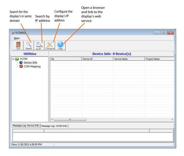
Click on COM Mapping to display the COM Mapping page, shown below. The controls on this page allow you to make virtual COM ports and select the display to which you want to map each virtual COM port.
