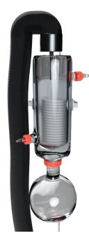
Engineered specifically for use with rotary evaporators, our revolutionary Bent Probe Immersion Coolers change the way your lab is organized. By allowing for the probe to hang directly on the edge of the glass condenser, no additional space or support is required.
