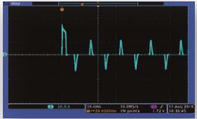
Inrush Current for 90° Start Angle
