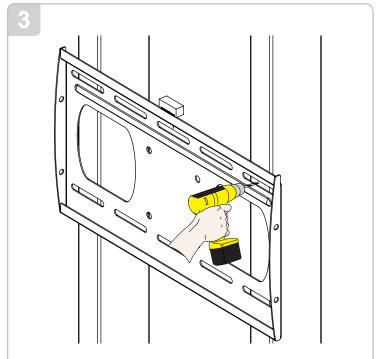
Drill a "pilot hole" in the center of the upper right mark using a 1/4" drill bit and power drill.
