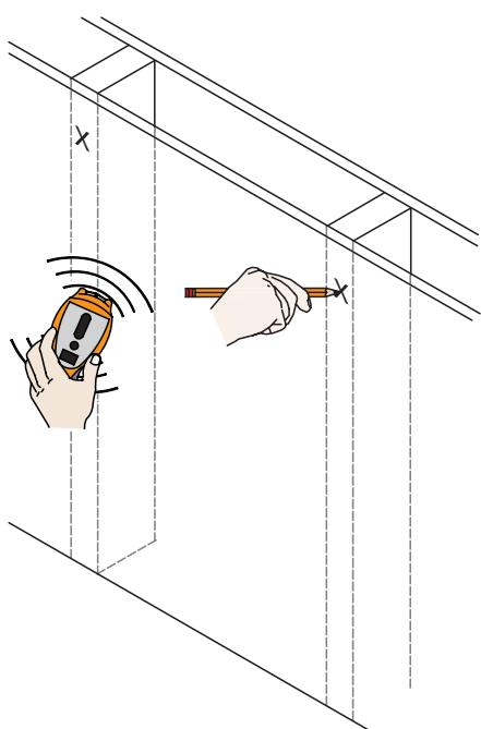
**!** You must secure the wall plate to two (2) wall studs with a minimum of four (4) lag bolts (2 lag bolts for each stud found).
