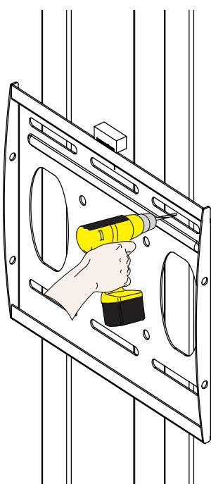
Drill a "pilot hole" in the center of the upper right mark using a 1/4" drill bit and power drill.
