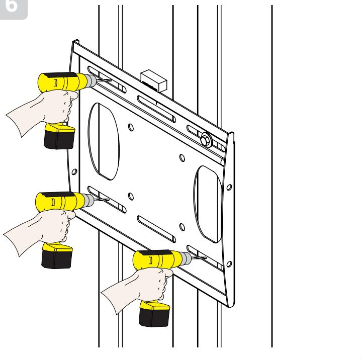
! Two people are recommended for this step; one person to level the wall plate and another person to drill the pilot holes.
