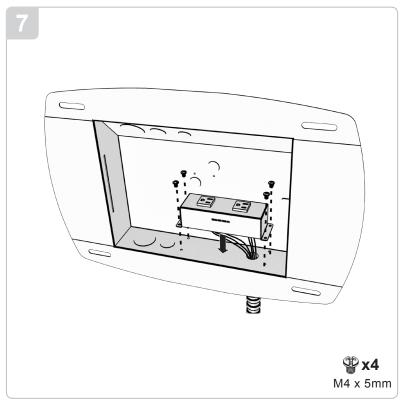
Firmly attach the A/C power box to the in-wall box frame with the four (4) each supplied screws.
