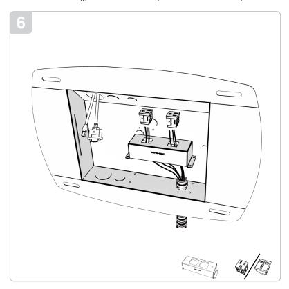
Attach the A/C power flex, Romex, and in-wall box frame, and hardwire directly to the two (2) each supplied "push in" A/C power replicates.
