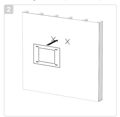
Use the 1/4" drill bit to create the initial hole along the trace line to insert the drywall saw.
