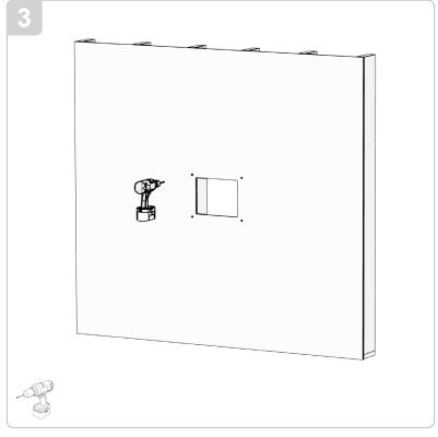
Caution: Make sure there are no exposed A/C wires or signal cables within the wall that might be cut while making the drywall cutout.
