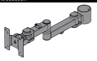
The MM-A1 is a single articulating multimonitor mount arm that works with any 2" tube. The mounting head provides 90° of omnidirectional tilt. and include both 75x75mm and 100x100mm VESA mounting patterns. The arm includes integrated cable management tabs to keep wires and cables protected and organized.
