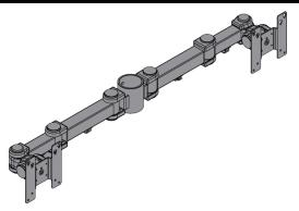
The MM-A2 is a dual articulating multimonitor mount arm that works with any 2" tube. Each mounting head provides 90° of omnidirectional tilt. The mounting heads include both 75x75mm and 100x100mm VESA mounting patterns. The arm includes integrated cable management tabs to keep wires and cables protected and organized.
