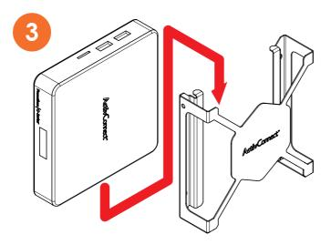
Orientate the ActivConnect as shown when mounting on an ActivPanel
