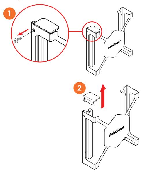
Orientate the ActivConnect as shown when wall mounting the bracket
