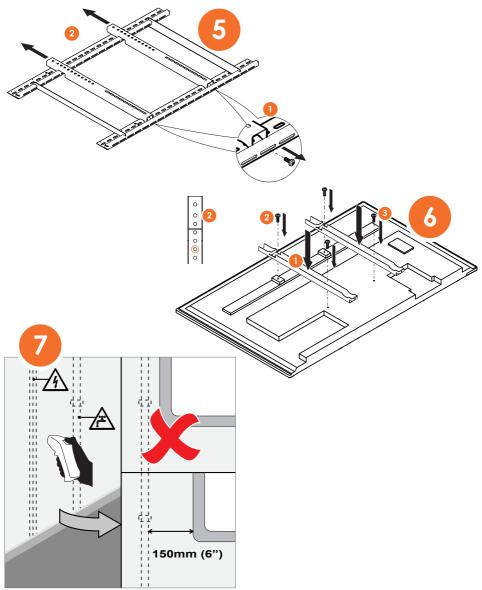
Use applicable device to detect hidden pipework in the wall
