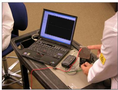
Measure, Record, Analyze & Report Electrostatic Voltage Generation and Decay
