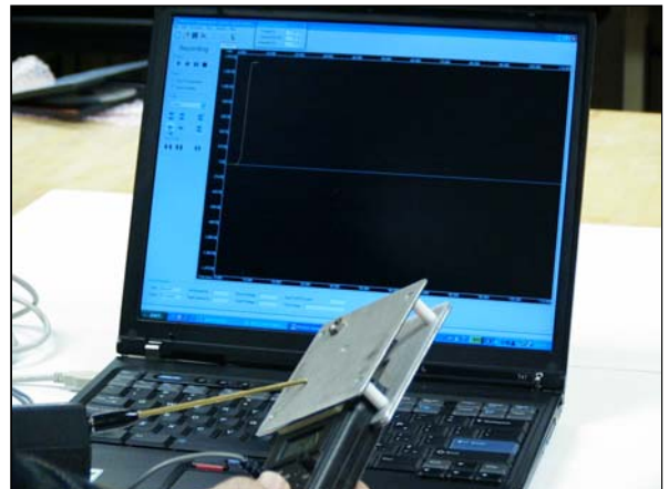
Figure 50: Charging the Charge Plate Monitor (CPM) to > 1,000 Volts
