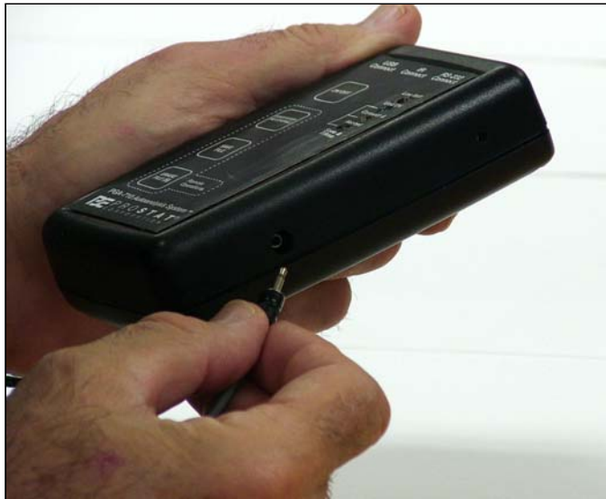
Figure 3: Connect Field Meter Output to Autoanalyzer input
