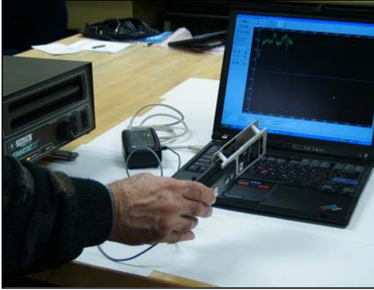
Figure 48: Making Offset Measurements on Bench Top Ionizing Blowers
