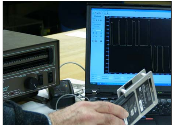
Figure 51: Performing Decay Tests on Bench Top Ionizer
