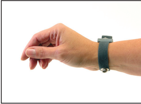
Figure 1: Attach Wrist Strap to test hand
