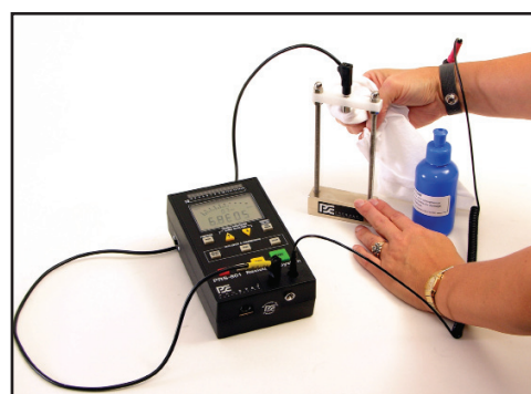
Figure 6: Clean electrode with alcohol
