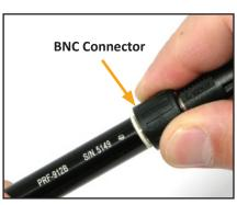
Figure 2: Connect shielded cable to PRF-922B's BNC fixture
