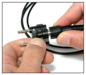
Figure 3: Connect Cable to Banana Converter
