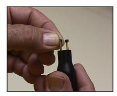
Figure 9: Installing Conductive Rubber Electrode "Boots"
