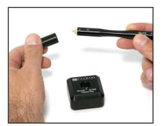
Figure 5: Remove Probe Cover
