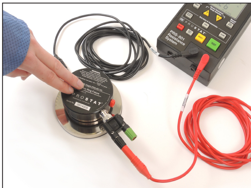
Figure 8: Confirming Electrode Contact to Test Bed
