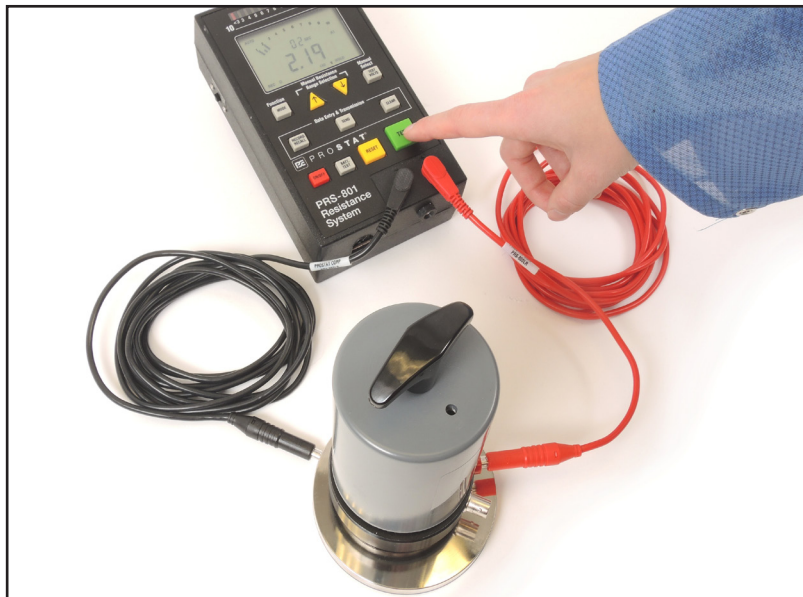
Figure 9: Confirming Electrode Contact to Test Bed
