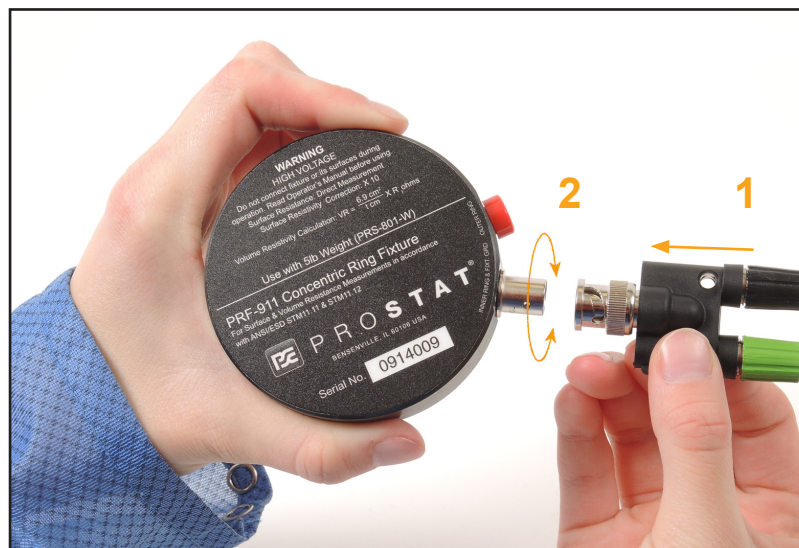
Figure 4: Installing the BNC Adapter
